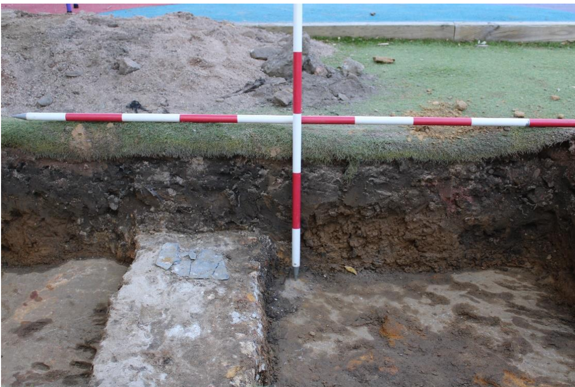
Figure 5-13. Test Trench Two stratigraphic profile with exposed bedrock at base, facing west (Jacobs 2024)
